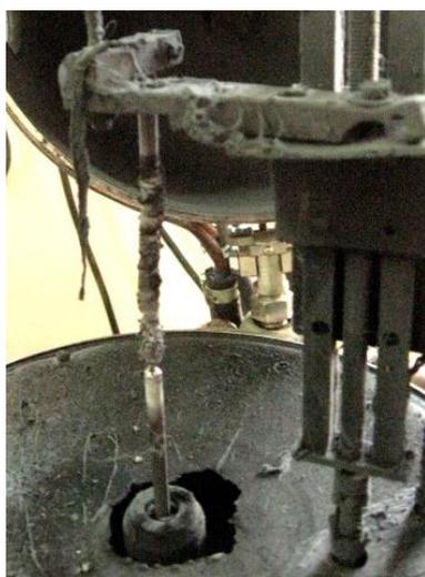
*Fig. 2 – Photo of electrodes (cathode with CD on top of it) after 5 cycles of arc discharge*
