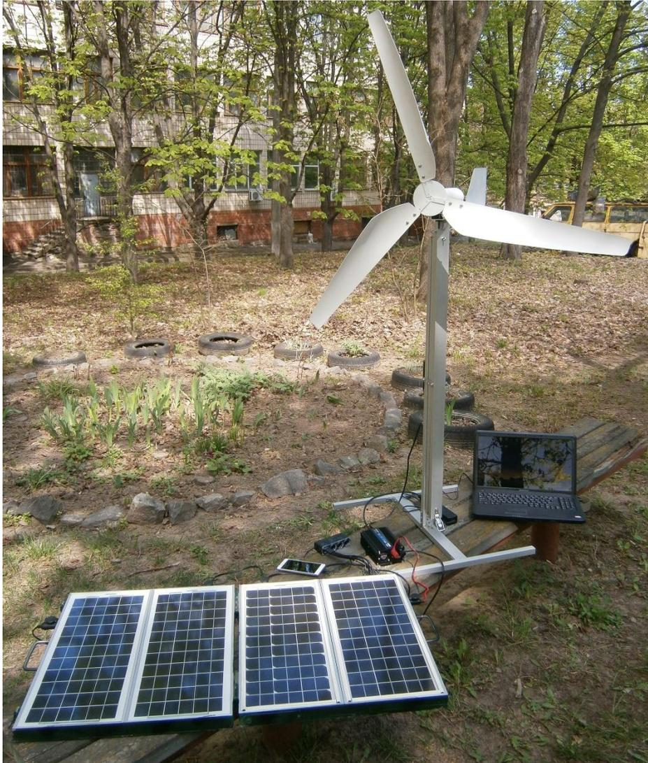
*Fig. 2 – Appearance of mobile combined photovoltaic / wind power station in its “working” state*
