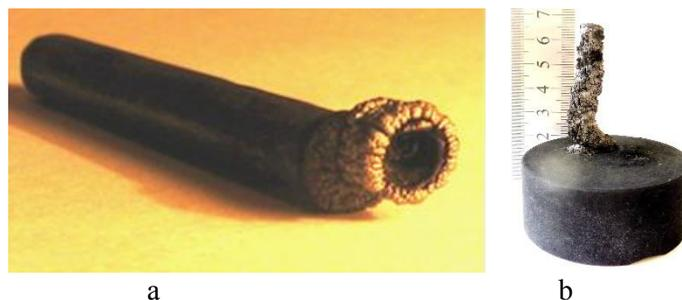
**Fig. 4** – The CD photo: a - cathode D 6 mm, anode D 6 mm; b - cathode D 50 mm, anode D 6 mm
