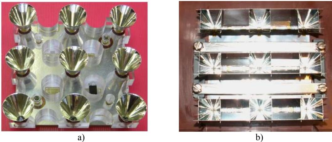
**Fig. 1** – Receivers of concentrated solar radiation based on triple-junction gallium-arsenide SC with types of integrated secondary optics: a) truncated cone, b) truncated pyramid
