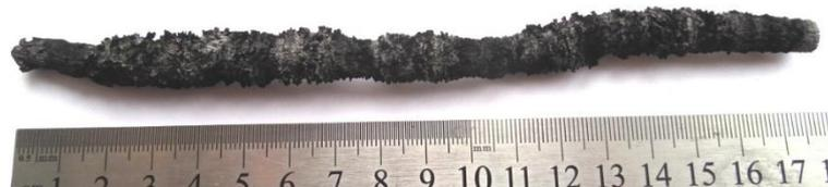
**Fig. 3** – Photo of 180 mm long cathode deposit obtained by ablation of an anode 6 mm in diameter
