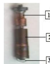
Fig. 2. The tunnel diode module in coaxial line: 1 is the piston with adjusting wheel; 2 is the section of short-circuit coaxial line; 3 is binding loop of the tunnel diode with cavity.
