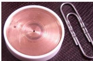
Fig. 3. The coplanar system of ring measuring electrodes - Corbino system. It consist the (in radial direction): inner disc is electrode to LF amplifier (or bridge), the separating ring at the ground potential, outer measurement ring - to LF generator signal, guard ring for forming the surface electron spot, the insulated ring
